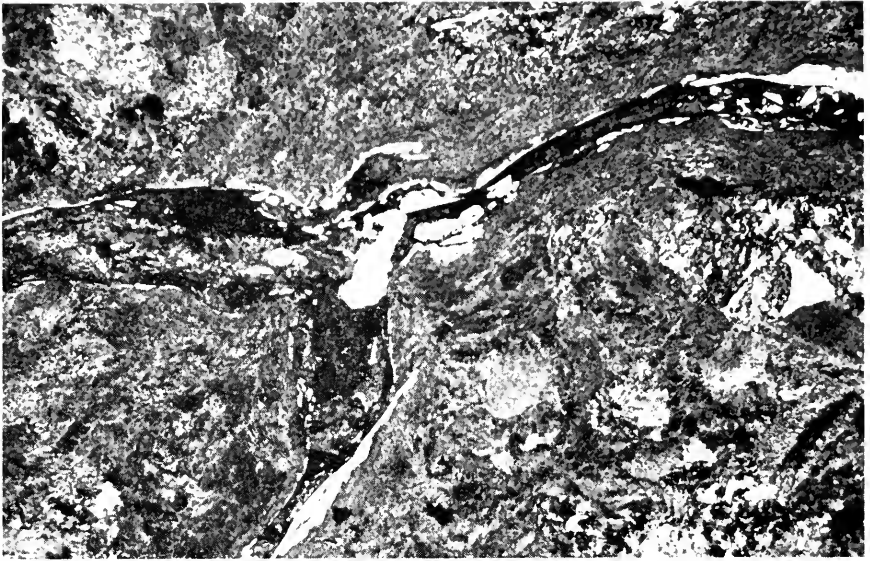
Fig. 5 (Investigation 132-10B)—Photomicrograph showing a different area of the same shelly crack shown in Fig. 4. Magnification, 250X. Etchant, 3 percent nital.
